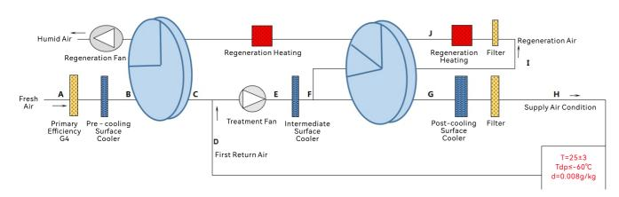
The low - dew - point dehumidification series adopts a "dual - stage dehumidification wheel + three - stage surface cooling dehumidification" system design. With high - quality sealing materials, a well - thought - out structure, and a proprietary smart control system, it can lower the dew point of the supply air at the unit outlet to -70°C. This meets the temperature and humidity control requirements of all production process stages in different areas of lithium - battery workshops.
