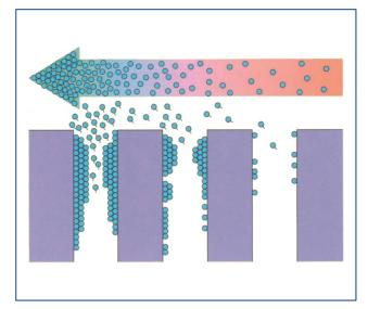
Heated regeneration air is fed into the regeneration zone from the back. The water molecules adsorbed in the silica gel micropores are activated by the temperature rise, weakening the adsorption force. Consequently, the water molecules flow out of the silica gel micropores.
