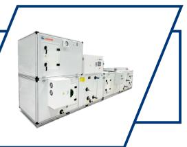
The low - dew - point dehumidification series adopts a "dual stage dehumidification wheel + three - stage surface cooling dehumidification" system design. With high - quality sealing materials, a well - thought - out structure, and a proprietary smart control system, it can lower the dew point of the supply air at the unit outlet to -70°C. This meets the temperature and humidity control requirements of all production process stages in different areas of lithium - battery workshops.
