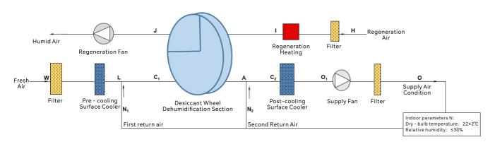
The desiccant wheel dehumidification section can handle an air volume of 1000~50000 CMH. When paired with OBAIR modular air - handling units or direct - expansion air - handling units, it can reduce the relative humidity of the air to below 30%RH, while ensuring indoor cleanliness, temperature and humidity, and air flow rate control requirements.
