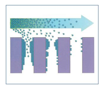
Water molecules in the air are absorbed by hydroxyl groups in the micropores of silica gel. Also, capillary condensation in the micropores absorbs much water from the air.
